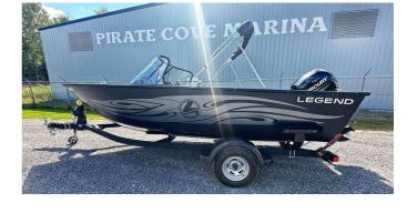
The 2019 Legend F19 was a crossover fishing and ski-style boat with a deep-V hull, a 94-inch beam, 42-inch hull depth, and a maximum 150 horsepower engine. It featured large bow and stern casting decks, multiple storage compartments including a rod locker, a live...
