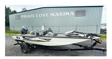
The 2021 G3 Sportsman 1610 is a 16' 10" fishing boat with an aluminum hull, a maximum 70 hp engine, a 64-inch beam, and a 1066 lb dry weight. It features a spray-in liner, large storage boxes and a generous casting deck. The boat has a 21-gallon fuel capaci...
