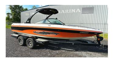
The 2006 Malibu Wakesetter 21 LX is a 21-foot wakeboard boat with a beam of 98 inches and a draft of 27 inches. It can carry a maximum of 12 people and has a fuel capacity of 50 gallons. The boat weighs approximately 4,580 lbs dry and can handle a we...
